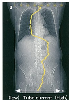
Visually grasping the variation of a tube current
